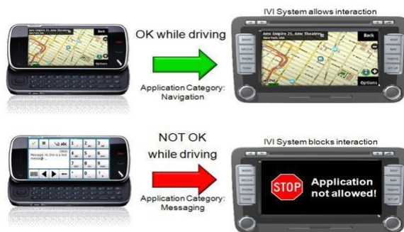
Figure 10. Preventing Driver Distraction
