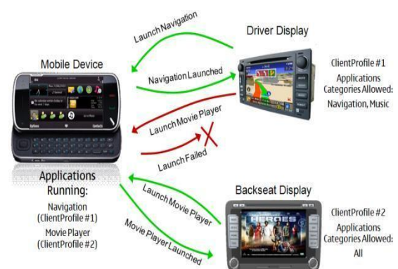
Figure 7. IVI System using Multiple Client Profiles
